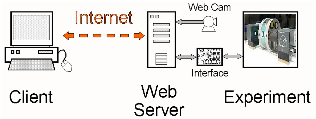
**Fig. 1:** Principle of a remote lab: A user with client computer controls a real experiment at a remote location via Internet. The experiment is controlled by the user through a web server and an interface; at least one web cam allows the user to observe the experiment and to take data.
