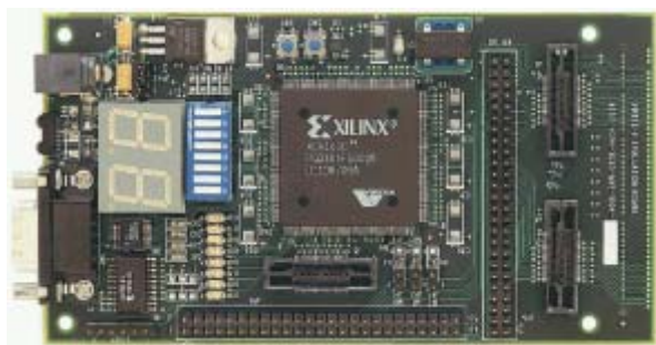
Figure 3: The FPGA board used to support hardwired logic experiments.
