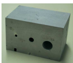
Real test piece of aluminium with different bore holes
